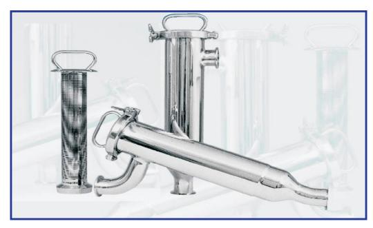
Memtech's 316L stainless steel filters are designed to remove suspended solids from fluids with particular application to the Food, Dairy, Brewing, Beverage, Pharmaceutical and Chemical industries. Their robust wedge wire elements are fully interchangeable and are available in standard micron elements from 10 to 1000. The units can be backwashed for cleaning which gives high security against breakthrough.
